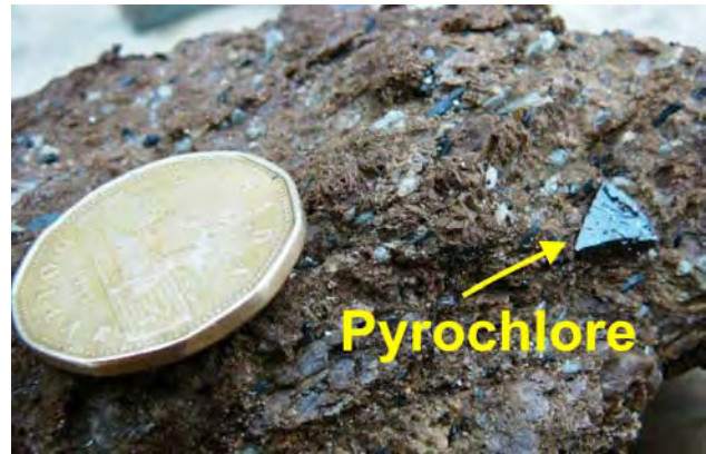
Figure 4.9. Pyrochlore expressing prominently in a sample of weathered carbonatite at the Blue River Tantalum and Niobium project.
