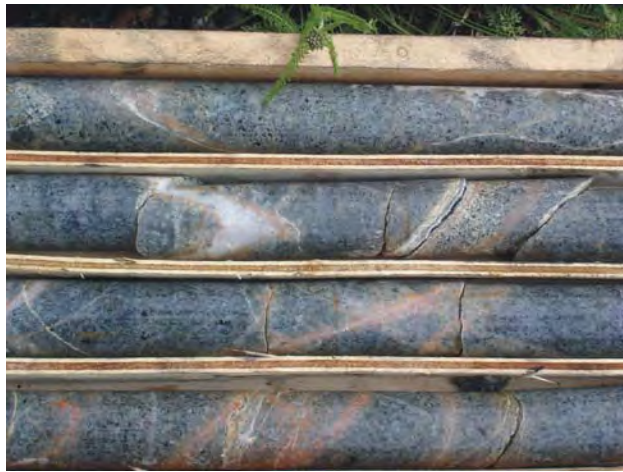
Figure 1.33. MO property, quartz-molybdenite veins with pink K-feldspar envelopes.
