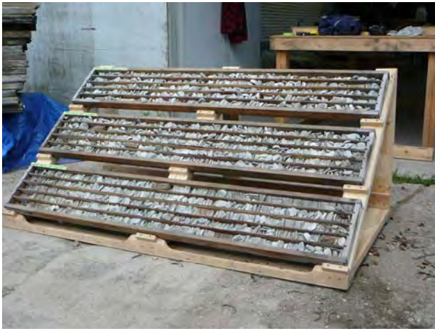
Figure 4.13. Old core being readied for re-logging at Yellowhead Mining Inc's Harper Creek project near Vavenby.
