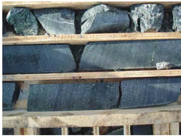
Figure 1.42. Aspira, wispy disseminated pyrite (and sphalerite) in mafic meta-volcanic rock.
