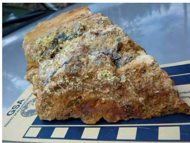
Figure 4.12. Sample of molybdenite-bearing quartz vein in a float sample at the Crazy Fox property of Newmac Resources Inc near Little Fort.
