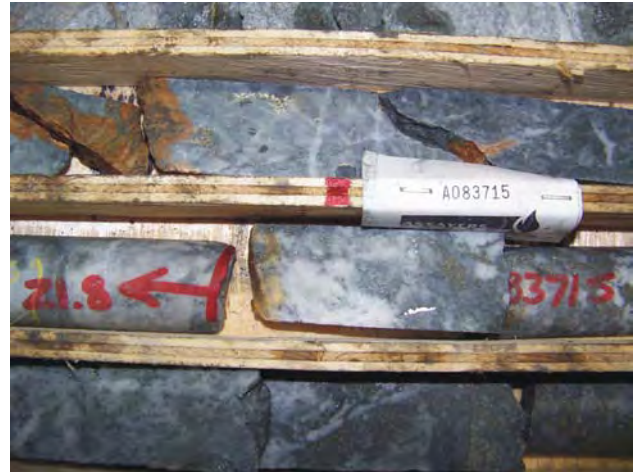
Figure 1.50. Dilworth, native silver and pyrite in quartz vein breccia from the Snow zone.
