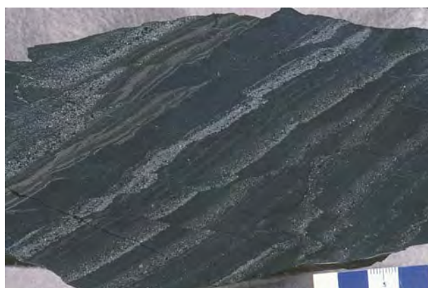
Figure 1.5. Eskay Creek ore, sulphide – sulphosalt mineral layers in mudstone. Note small-scale offset on cleavage fractures.
