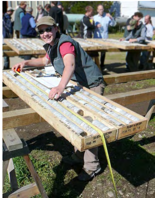
Figure 4.10. Drill core logging at the Blue River Tantalum and Niobium project of Commerce Resources Corp.
