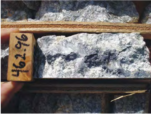
Figure 1.36. Lone Pine, quartz-molybdenite vein in the Alaskite zone.
