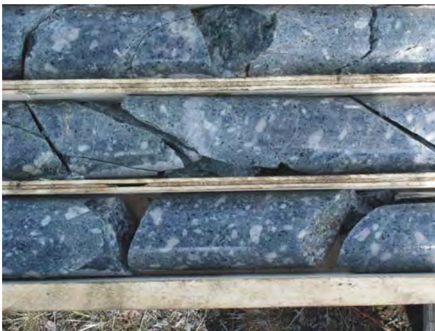
Figure 1.30. Swan, a porphyritic phase of the Glundebery batholith in drill core, with prominent potassium feldspar.
