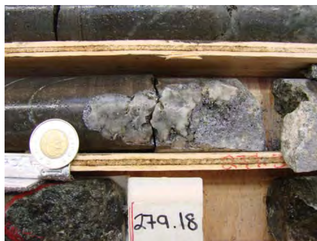
Figure 3.13. Molybdenite selvage with quartz in argillite, Chu project.
