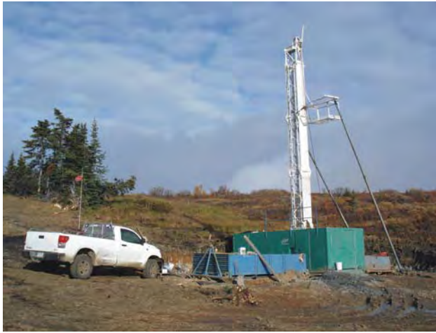
Figure 1.19. Red Chris, Boyles 56-model drill, capable of drilling to 1500 m.
