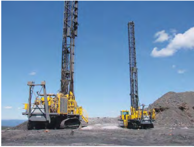
Figure 2.5. New “Pit Viper” blast hole drills at the Trend Mine.
