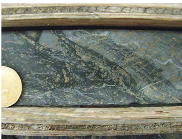
Figure 3.11. Drill core grading 33 g Au/tonne, Main Zone, Spanish Mountain.
