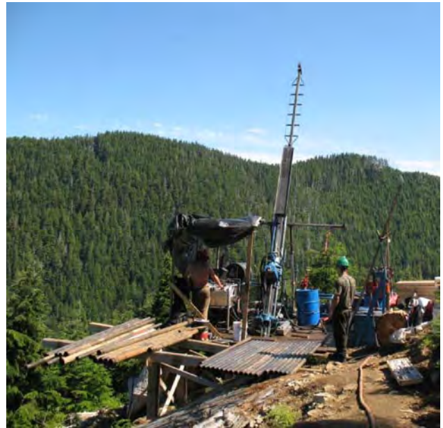
Figure 5.9. A helicopter-portable drill rig on the Cliff zone at Catface Copper.
