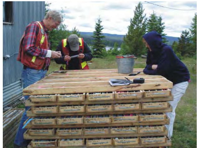
Figure 1.56. Nechako, inspecting drill core.
