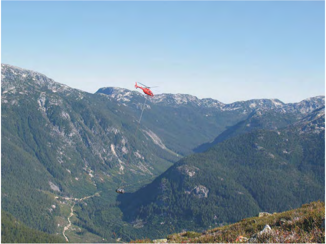
Figure 5.13. Slingshotting with a long line at the Crack molybdenum project. Despite an extensive road network, the rugged terrain (and road deactivation) necessitated helicopter support for several projects on the east side of Harrison Lake.
